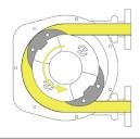
When the pressing shoe in the outlet direction leaves the hose, the other pressing shoe is already compressing the hose, so as to avoid internal backflow leakage, and then suck the medium in sequence with the movement of the wheel.
